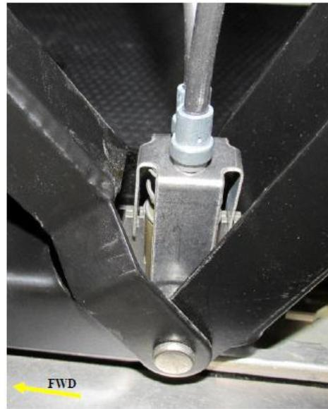
Undamaged Locking Foot Cap
