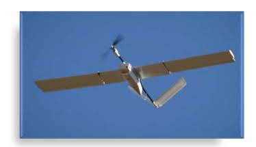
The Falcon is classified by the FAA as a "small" UAS as it weighs less than 55 lbs. (actual weight is approximately 12 lbs.). The pilot launched the aircraft and placed it in "auto" mode (autonomous navigation) in order for it to accurately fly its mapping profile. The operating altitude was approximately 200 meters (656 feet) above ground level (AGL).
