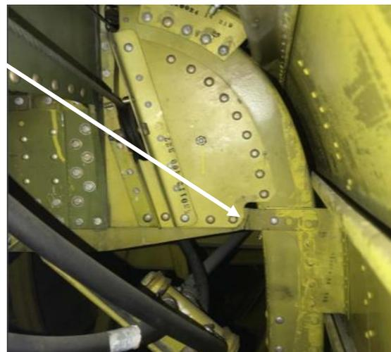
The cracks in the third Aero Commander progressed much further than the other two (Figure 4). This area lies within the bulkhead area forward of the vertical fin attachment bulkhead.
