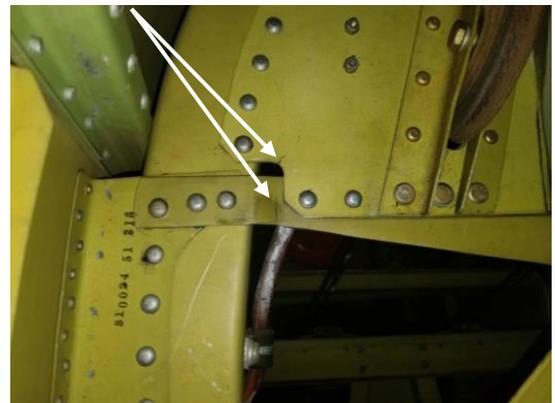
Figure 2 and 3. Cracks in aircraft bulkhead.
