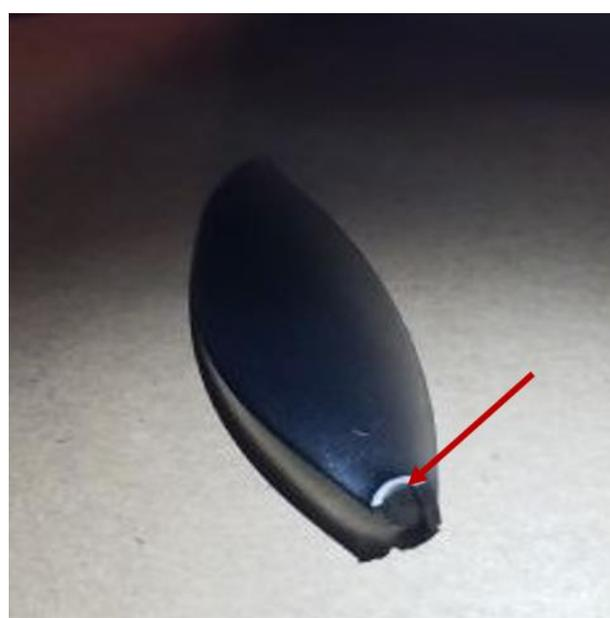
A civil online forum addressed the issues associated with the Anafi Parrot propellers. They noted that markings (dings) and cracks can develop when the propeller contacts the mounting for the other propeller upon startup. According to the forum members, a “best practice” would be to change the propellers between every 100 and 120 flights in order to mitigate the risk associated with the loss of propeller blades.
