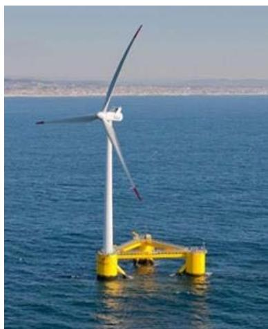
**A full-scale prototype of the WindFloat device**
