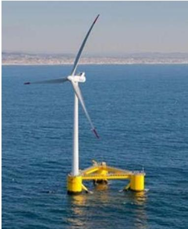
**A full-scale prototype of the WindFloat device**
