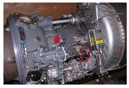
concerns that this condition could be present in other aircraft with this particular engine type. Ultimately, this could allow the stator vane assembly to move and contact the rotating compressor. Compressor stalls could result from the bolt binding in the mount hole and preventing bleed band closure.
