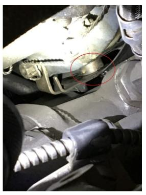
Retainer bolt and lock cup pictures in the 2 o'clock position. Hardware is also installed in the 4, 8, and 10 o'clock positions.
