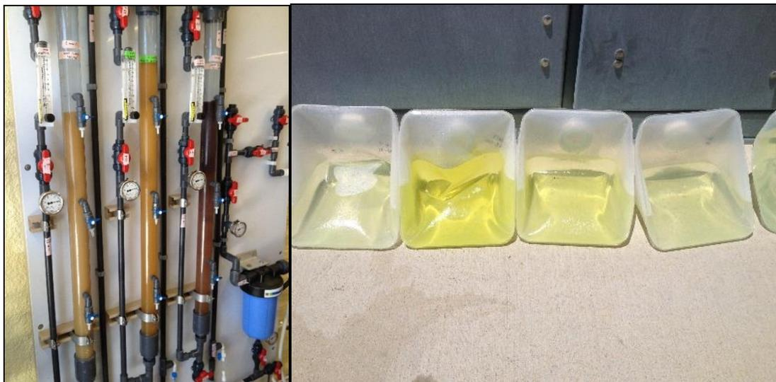
Left: Pilot-scale ion exchange resin columns. Right: Regeneration brine. [Photo credit: Reclamation].
