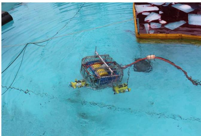
The skimmer prepares to submerge and maneuver under the containment skirt to recover the oil. [Photo credit: BSEE].
