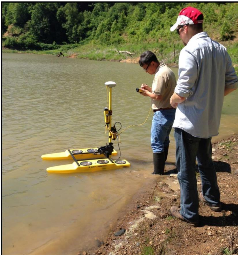
OSMRE staff preparing the bathymetric survey equipment for use in an impoundment at a coal mine in Tennessee. [Photo credit: Stefanie Self, OSMRE].
