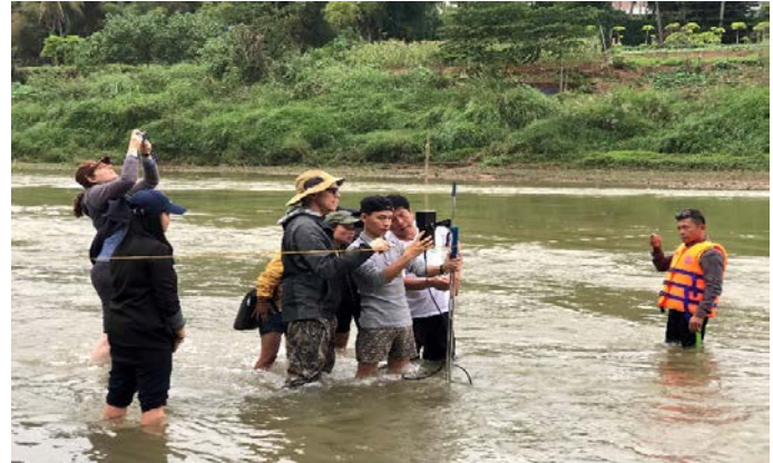
DOI technical expert demonstrates the operation of the hand-held flow meter during a Basic Hydrology and Measurements Training, Lao PDR, January 11, 2018
