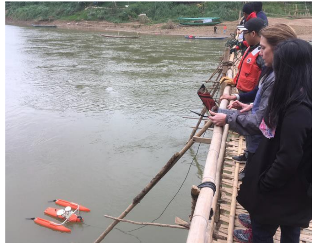
DOI technical expert demonstrates how to measure discharge with an acoustic Doppler current profiler. Luang Prabang, Lao PDR, January 11, 2018 Credit: DOI-ITAP, Kulthida Techasarin
