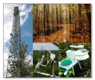
Instruments used to measure carbon fluxes in air, soil, and water help gain understanding of how carbon is stored and transferred within different ecosystems, which is critical to effectively managing carbon sequestration. Image source: USFWS.
