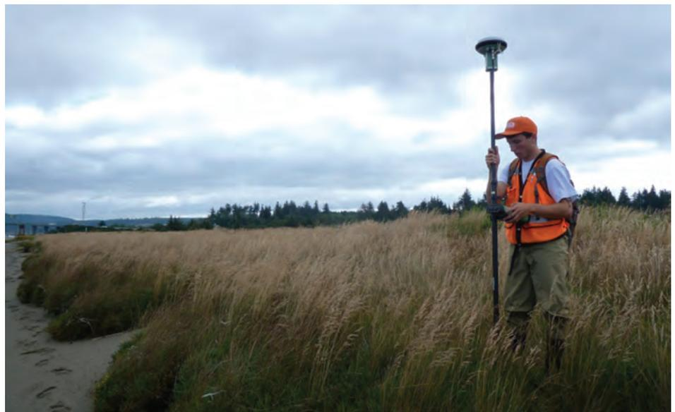
A USGS technician collects critical elevation data using a Real-Time Kinematic Global Positioning System at the Bandon National Wildlife Refuge, managed as part of the Oregon Coastal Refuge Complex, in southern Oregon. Photo credit: Katherine Powelson, USGS
