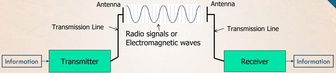
The transmitter generates a wireless signal based on the information and feeds it to an antenna by a transmission line
