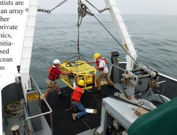
USGS scientists and staff deploy a camera sled from the research vessel *Shearwater*. The sled is towed close to the seafloor and collects realtime photographs and videos. On board the vessel, scientists can watch the live video feed and make note of seafloor characteristics such as sediments, rocks, and biological cover to enhance the California Seafloor Mapping Program offshore of northern California. Photo credit: USGS
