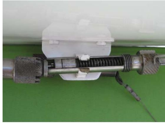
Figure 4 Manual Release Mechanism (cover removed)
