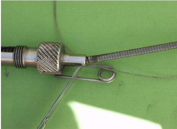
Figure 3 Damage to manual release cable
