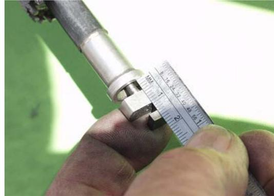
Figure 8 Gap in comparison cable
