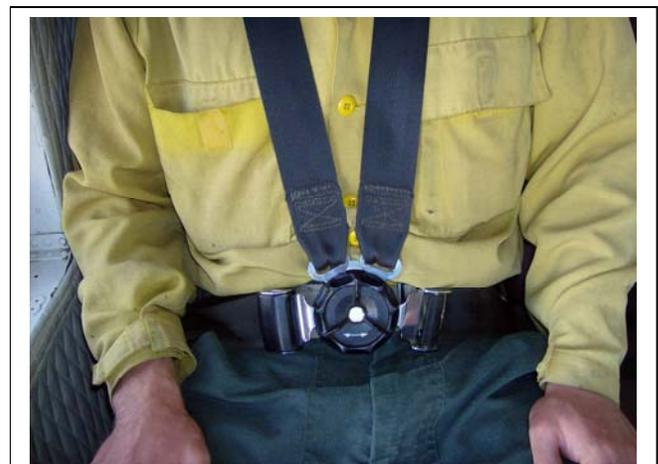
Figure 1 - Seat Belt correctly fastened
