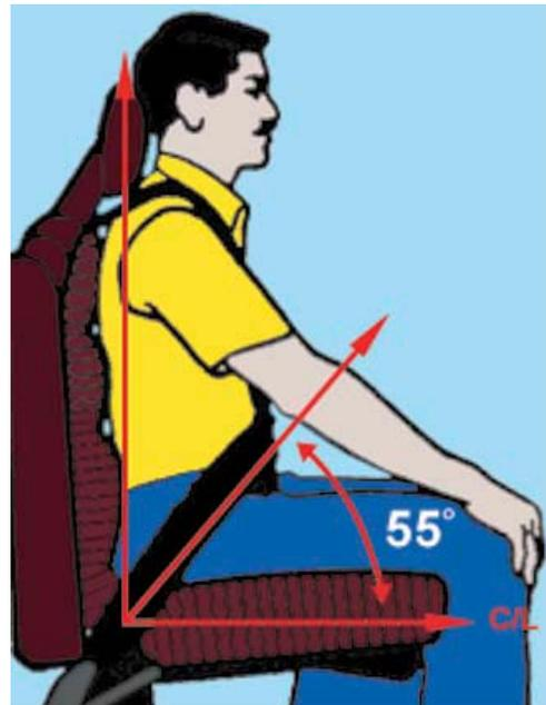
Figure 3 - The safety belt should be positioned so that it makes an angle of about 55 degrees with the centerline of the aircraft.
