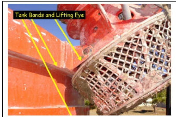
**Portable Retardant Tanks.** The frame of portable retardant tanks (PRT) may have lift rings, tank bands (aka collars), or other structural components that can “catch” snorkels and water buckets. All PRTs should be inspected, and any structural hazards mitigated, prior to use.
