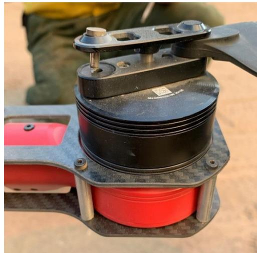
Figure 3 – New style prop shear.
