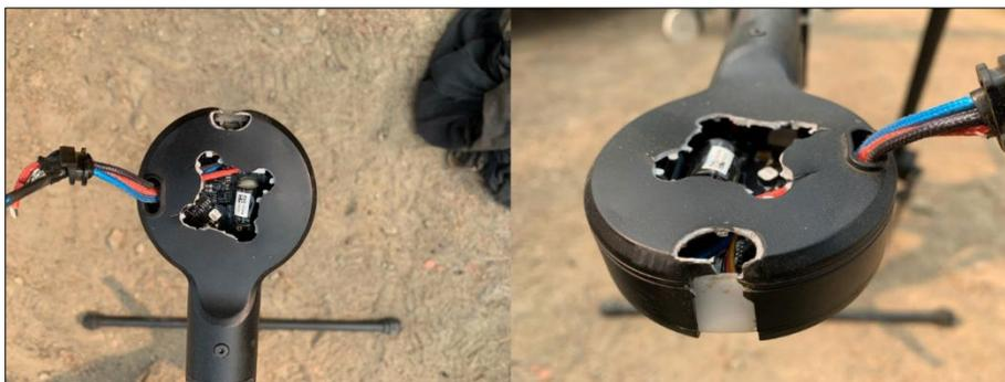
**Figure 2: Motor mount after departure of motor.**
