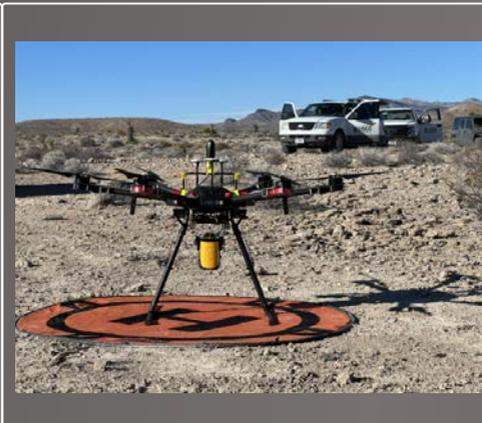
Lidar elevation map of the Great Sippewissett Marsh, Cape Cod, MA (left) and DJI Matrice 600 Pro with Lidar Payload (right).
