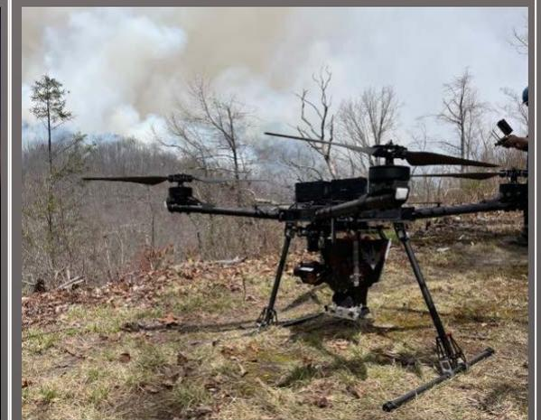
What's on the horizon for FY23? Interagency fire remained the top flight use category for UAS missions in FY22. The Freefly Systems Alta X with Droneamplified Aerial Ignition Payload (right). Photo credits: Steve Stroud, OAS.
