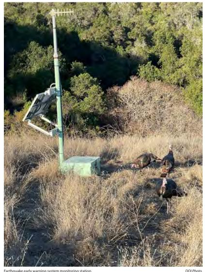
Earthquake early warning system monitoring station.
