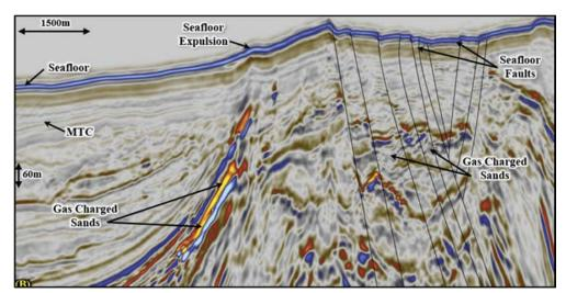
**Seismic Data Showing Shallow Geohazards** Source: https://ncs-subsea.com/seismic/applications/
