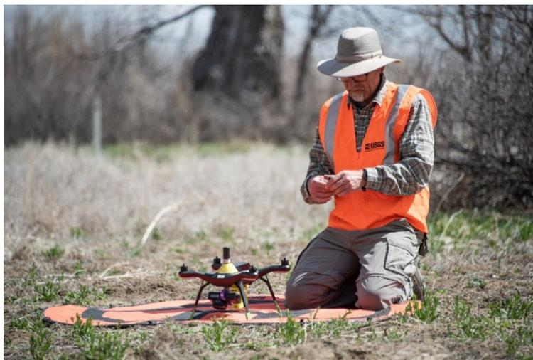
U.S. Geological Survey remote pilot Joe Adams prepares a 3DR Solo UAS for mapping, a mission dominated by this aircraft (Credit: M. Bauer).
