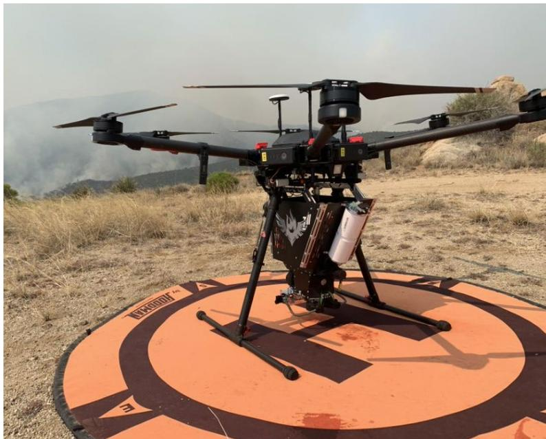
*The Drone Amplified Ignis payload has ignited DOI's utility for fighting wildfire with UAS. This Plastic Sphere Dispenser (PSD; shown here mounted to the Matrice 600 Pro Government Edition) provides firefighters the ability to build miles of fire-containing backfires in a short time, an activity previously conducted slowly on foot, or dangerously with a manned helicopter.*
