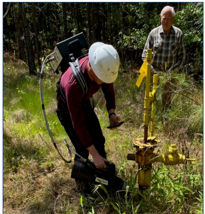
Figure 19: Louisiana contractor measuring methane emissions from a high emitting orphaned well in Union Parish, Louisiana.
