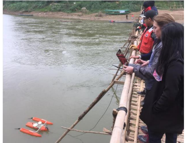
DOI technical expert demonstrates how to measure discharge with an acoustic Doppler current profiler. Luang Prabang, Lao PDR Credit: DOI-ITAP, Kulthida Techasarin
