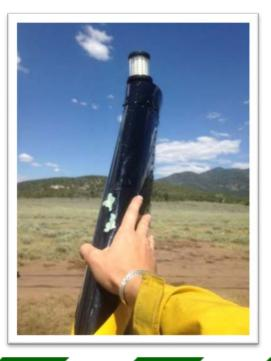
That afternoon while the helicopter was being washed, two dents were discovered on the vertical stabilizer fin six inches below the anti-collision light. They were approximately one inch wide and three inches in length with a depth ranging from 1/8 - 1/4 inch. It is believed that the sprayer used to wash the aircraft removed the paint chips that were covering the dents.
