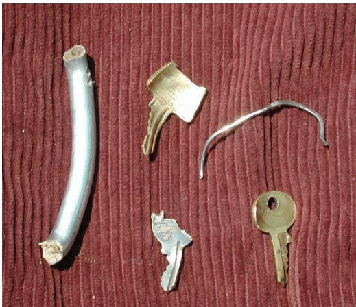
As soon as this occurred, the HMGB and pilot communicated the need to shut-down the helicopter. All personnel held positions until rotor blades were no longer turning. As soon as rotors stopped and it was confirmed that there were no injuries. They inspected and confirmed the rotor strike blade damage and located the mangled keys, key ring and carabiner. The pilot contacted the mechanic while the HMGB and helitack crewmember contacted dispatch and the COR to inform them of the mishap.
