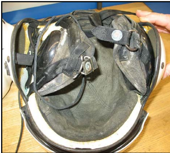
Figure 1. Mold and corrosion on the interior of this helmet poses a serious health risk.
