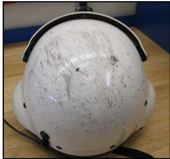
Figure 2. The deep gouge to the helmet's shell makes it unsafe and unserviceable .
