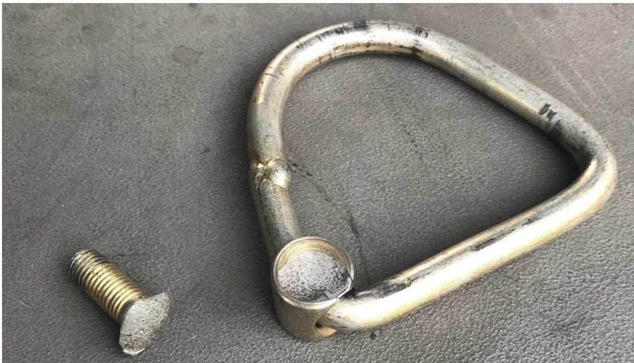
Figure 1 – Failed NAS1211B20 Ring and Stud Fitting
