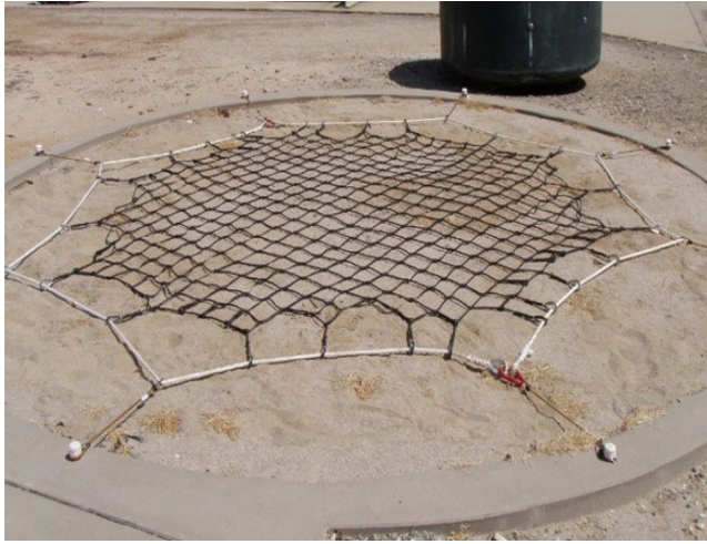
Figure 2 – Sample of NFES #000531 cargo net with perimeter rope attached correctly.
