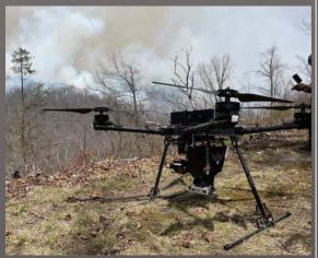
What's on the horizon for FY23? Interagency fire remained the top flight use category for UAS missions in FY22. The Freefly Systems Alta X with Droneamplified Aerial Ignition Payload (right). Photo credits: Steve Stroud, OAS.
