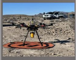
Lidar elevation map of the Great Sippewissett Marsh, Cape Cod, MA (left) and DJI Matrice 600 Pro with Lidar Payload (right).
