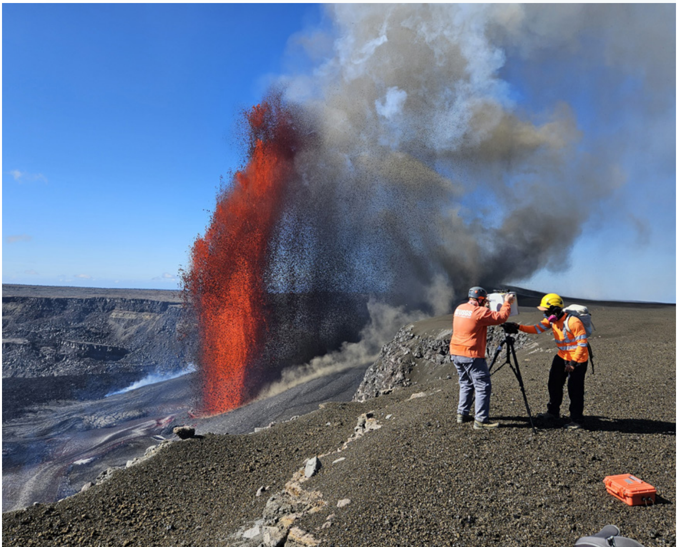
USGS scientists measure gas emissions during episode 28 of the Halema'uma'u Kilauea summit eruption.
