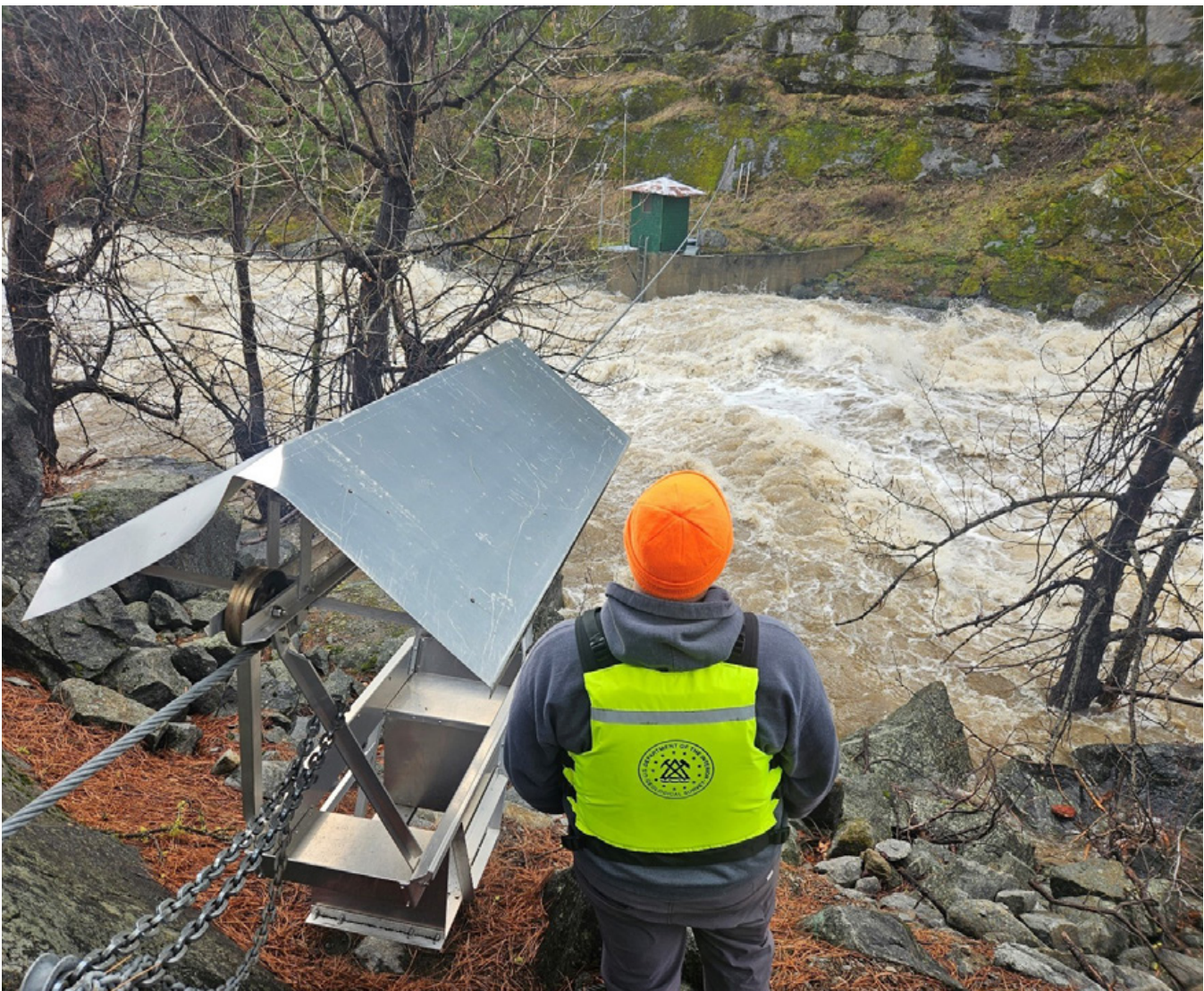
USGS technician preparing to make a streamflow measurement from a suspended cableway during historic floods at a USGS streamgage on Icicle Creek near Leavenworth, WA.
