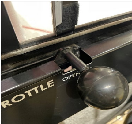
Figure 3. Notch in Throttle Panel
