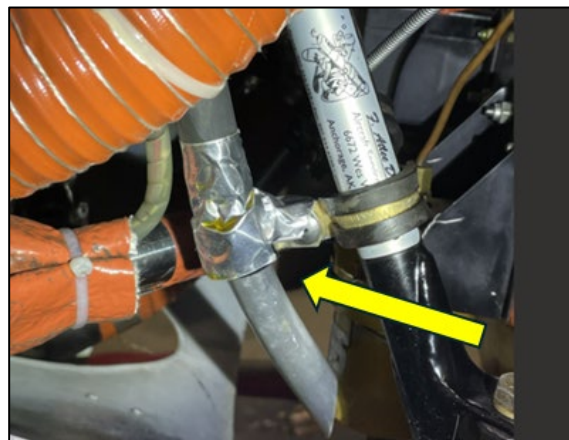
Figure 2. Oil Breather Tube Hole Taped Over
