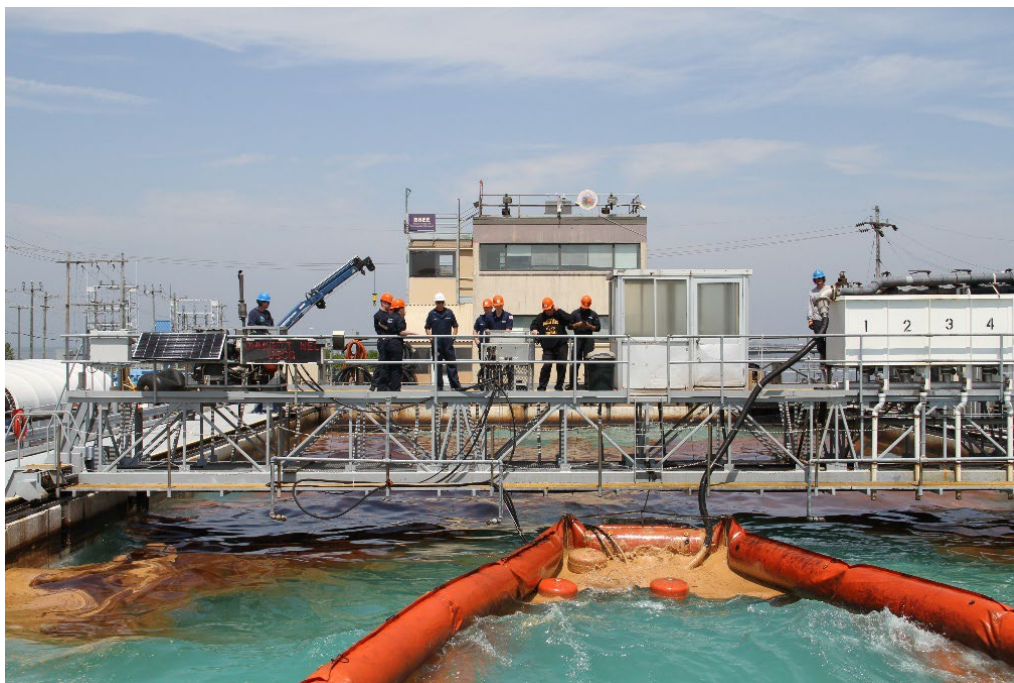
Figure 5. U.S. Coast Guard Strike Team personnel train on recovering oil with a skimmer in the Ohmsett tank. The USCG is an important customer for Ohmsett’s services.
