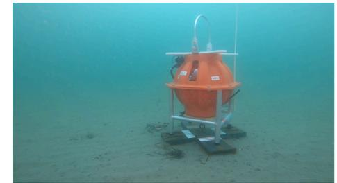
Testing small ocean-bottom seismograph deployed along the seafloor in Atlantic Ocean. Photo by Nathan Miller / USGS.
