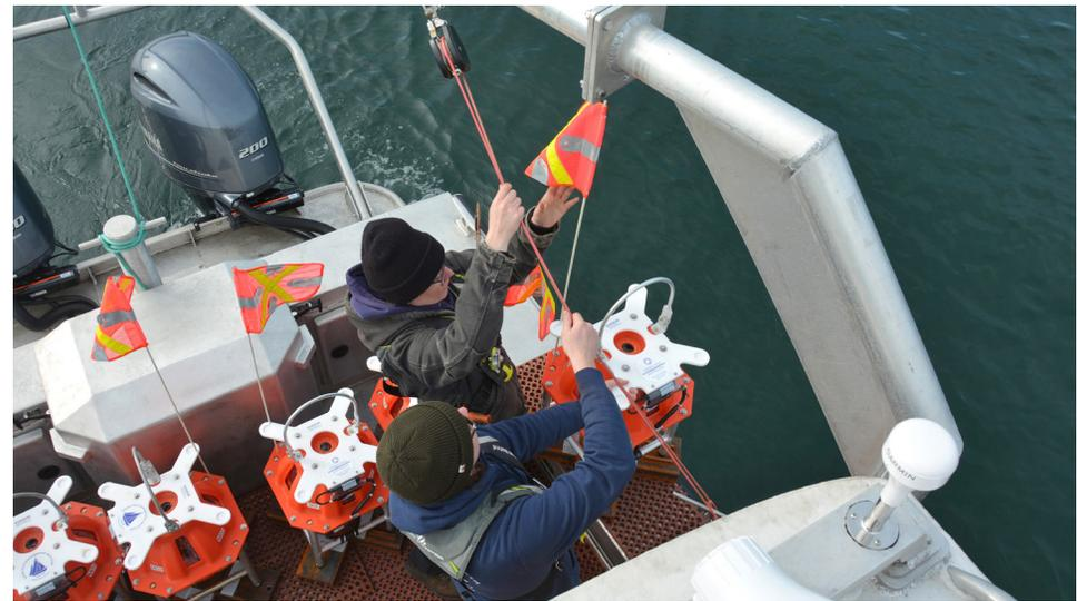
Collection of micro ocean-bottom seismometers ready to be deployed by the Weepecket Islands, off the coast of Massachusetts. Photo by Nathan Miller / USGS.
