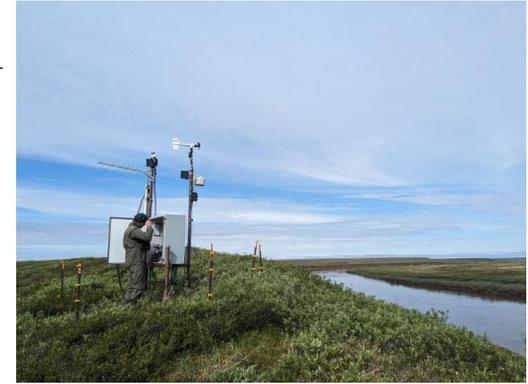
Ikpikpuk River gage setup: Meteorological sensors and data logger sit atop the west bank, with cables running to pressure transducers in the river to measure water depth. Photo by K. Drew.
