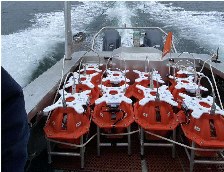
Small ocean-bottom seismographs being deployed in Atlantic Ocean to test their ability to be rapidly deployed. Photo by Nathan Miller / USGS.
