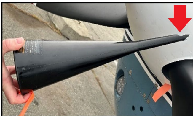
Figure 2 Long neck transmission funnel with cracked end.
