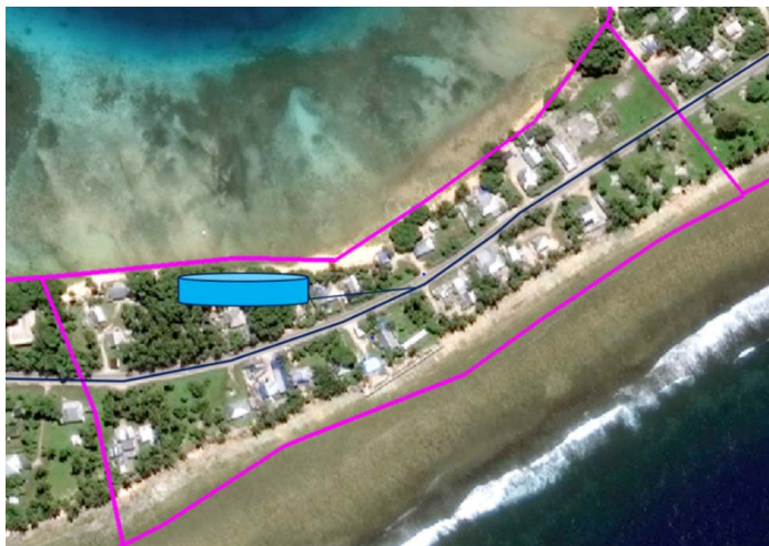
Figure 17: The same typical service area shown with one representative tank and distribution pipeline that is hydraulically equivalent. Pink lines indicate the boundary of modeled tanks and polygons.
