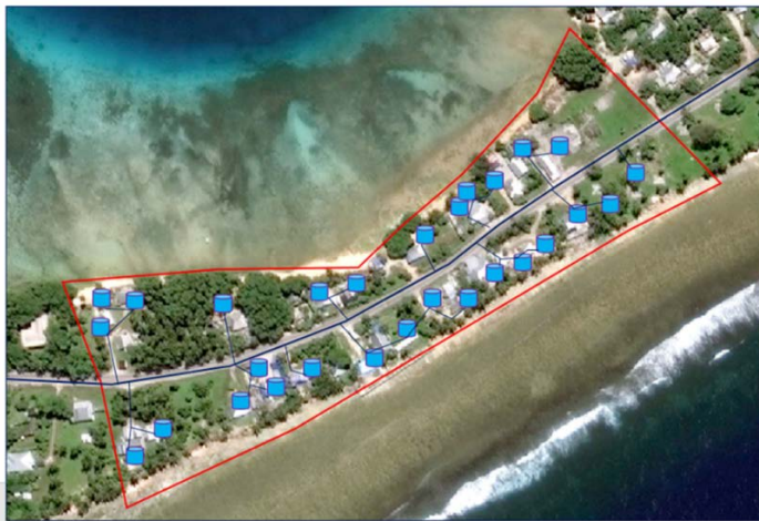
Figure 16: Sample of a single service area with multiple tanks and distribution pipelines served by the transmission main. Red lines indicate real tanks.
