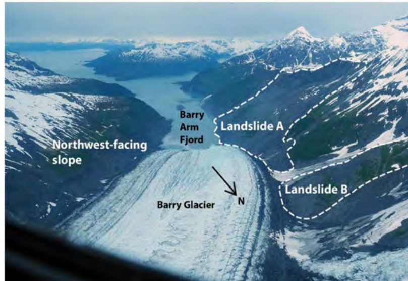
The USGS is working with Federal and State partners to assess the risk of a catastrophic landslide and tsunami at the terminus of a retreating glacier in Prince William Sound, Alaska. This photo shows the Barry Arm Fjord of Prince William Sound, the area of potential landslides outlined, and the retreating Barry glacier in the middle foreground. Photo taken by Gabe Wolken, June 2020 Source: Public domain.
