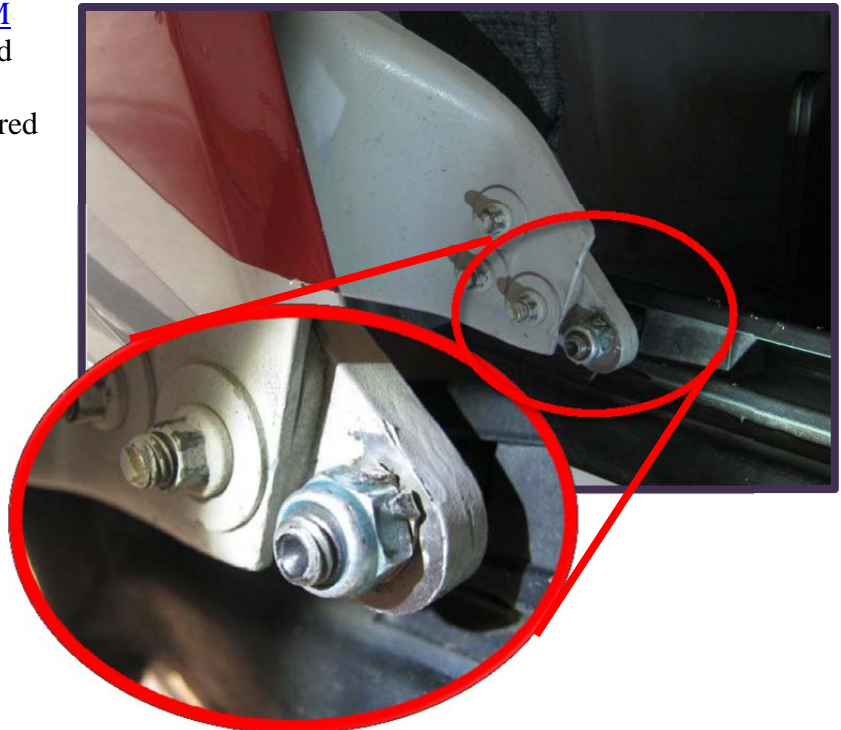
Figure 1 Right Hand Door Lower retention nut and lock-washer
