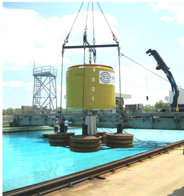
Figure 6. Wave energy harvesting technology tested at Ohmsett in 2013 by Seattle-based Oscilla Power, Inc. From: Fall/Winter 2013 Ohmsett Gazette . "Wave Energy Harvesting Technology Tested." Page 6. https://www.ohmsett.com/gazette.html .
